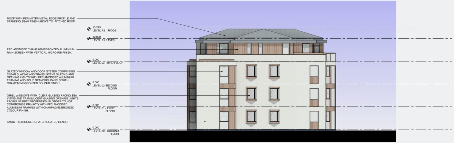
ROOF WITH PERIMETER METAL EDGE PROFILE AND STANDING SEAM FINISH ABOVE TO PITCHED ROOF.
