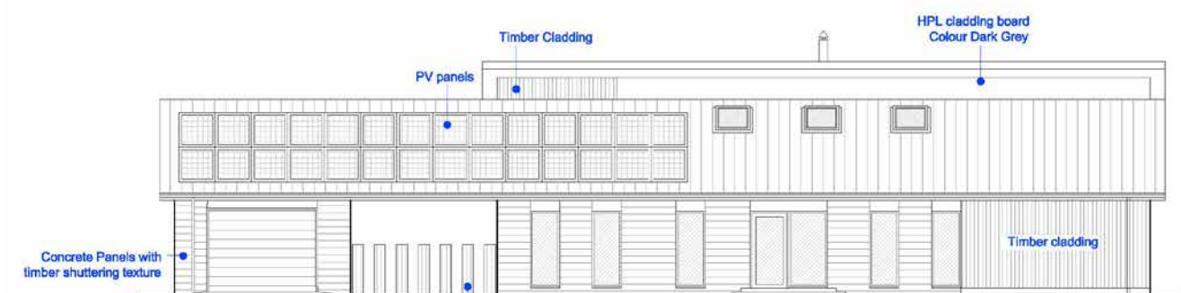
West Elevation (1:100 scale)
